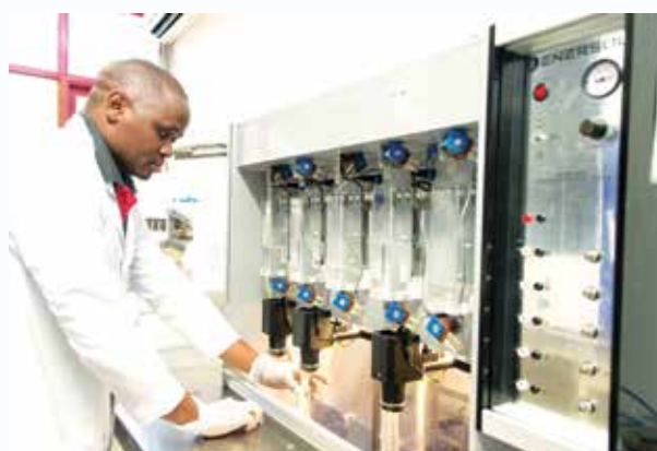
Engineer Peter Martin performs testing of condom samples in the Textile Laboratory.
